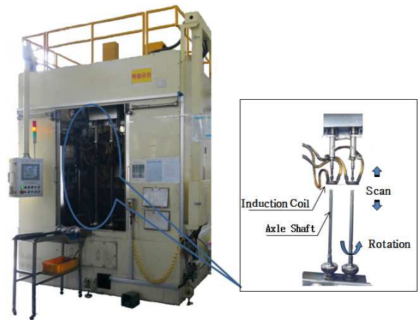
Fig. 3 Induction hardening shape and drive the structure
