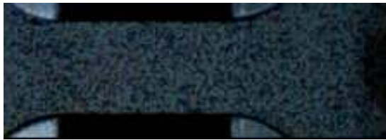
Fig. 4 Speckle pattern formed on the surface of the pure aluminum tensile specimen
