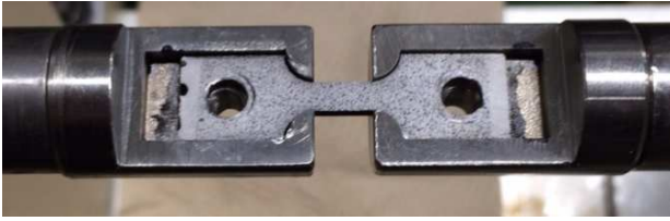
Fig. 3 Assembly of the tensile specimen and grips with adhesive
