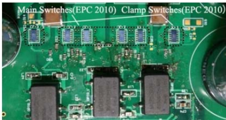
Fig. 8. PCB board of GaN FET based flyback-forward high gain DC/DC Converter.
