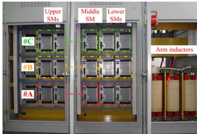
Fig. 9. Photograph of the laboratory setup.
