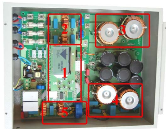
Fig. 10. System prototype: boost converter (2 strings)+ H-bridge converter: 1- TMS320F28069 board with control panel; 2- input filter; 3- boost converter inductors; 4- output filter; and 5- RFI filter.
