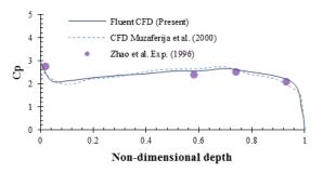
Fig. 8 Pressure distribution during water entry of arbitrary flare section at 0.07 s
