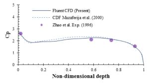
Fig. 9 Pressure distribution during water entry of arbitrary flare section at 0.08 s
