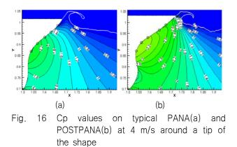
We summarized that POSTPANA with big bulb and large flare than the PANA's one suffers large impact pressure. At given impact velocity, the big bulb makes the several pressure picks at different places could be gathered at a moment and large flare also has bigger pressure on the arbitrary surface according to the simulation results.
