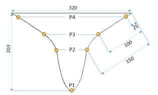
Fig. 1 Zhao et al. Experiment (1996) drop test section geometry (unit is mm)
