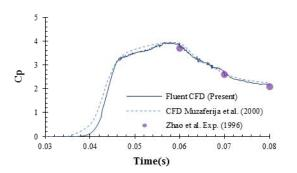
Fig. 6 Time history of pressure distribution at nondimensional depth  $\phi$  = 0.74 during water entry
