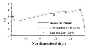
Fig. 7 Pressure distribution during water entry of arbitrary flare section at 0.06 s
