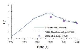
Fig. 5 Time history of pressure distribution at nondimensional depth  $\phi$  = 0.58 during water entry
