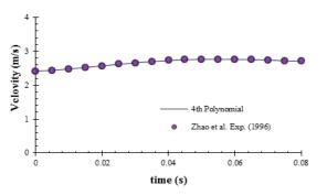
Fig. 4 Experimental water entry velocity profile of the arbitrary section
