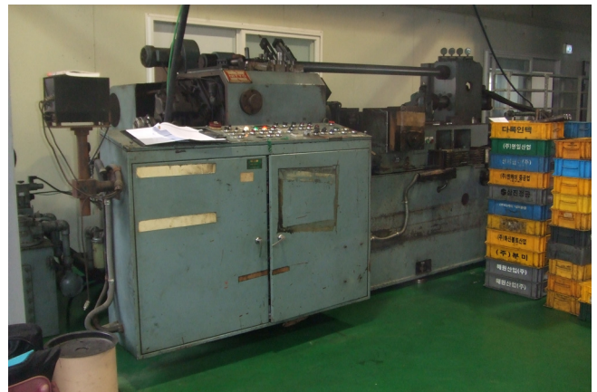
Fig. 3 Appearance of friction welding machine(Model: FF-60 II M-S1)
