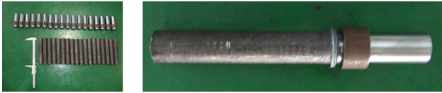
(a) Specimen of O.D. 36 mm (I.D. 25 mm) tube-to-tube welded (L = 315 mm)
