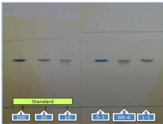
Fig. 2. TLC analysis of IAA produced from the selected strains. Concentration of IAA standard: 10, 30 and 100 \text{ mg L}^{-1} .
