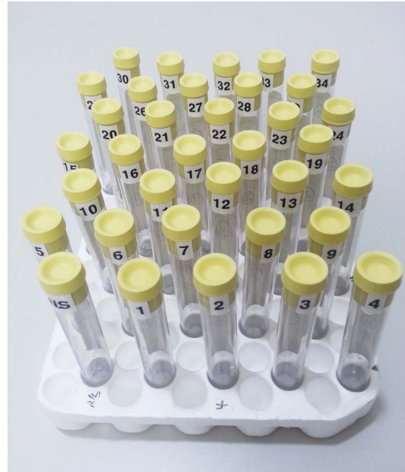
Fig. 2. (Color online) Self-construct phantom to evaluate molar concentrations.
