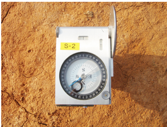
Figure 2. Clinometer as Archaeomagnetic sampling tool.
