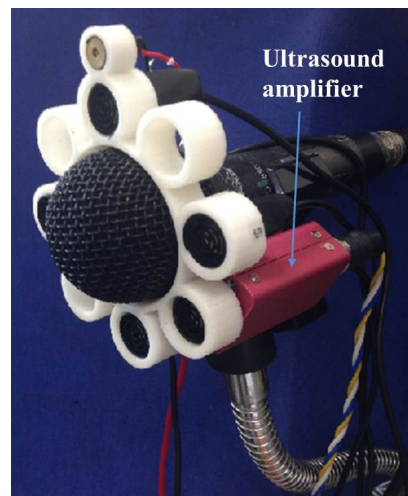
Fig. 3. The prototype acquisition equipment integrated with audio microphone.
