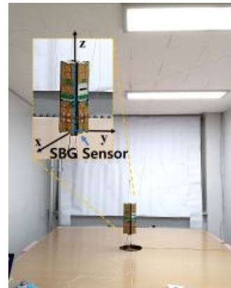
Fig. 16. Angular rate measure test setup
