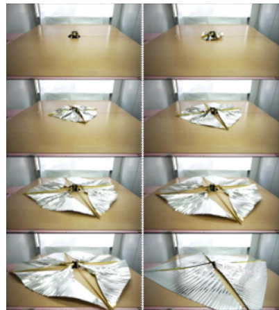
Fig. 13. Solar Sail Deployment ground Test
