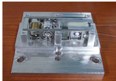
<Fig. 9> Prototypes of FBG Accelerometer
