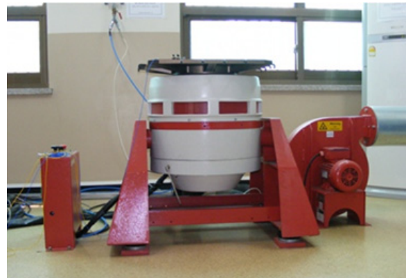
<Fig. 12> Vibration test equipment for the acceleration sensor with optical fibers
