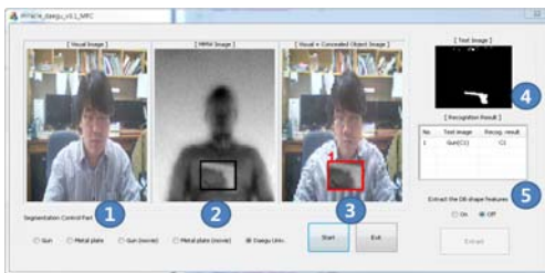
Fig. 6. MMW image segmentation of a gun and GUI display
