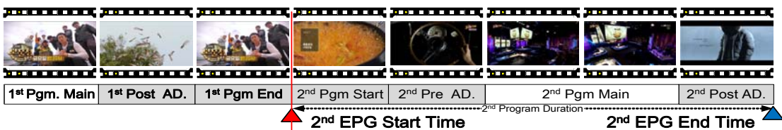
Fig. 10. EPG time information at the program connection
