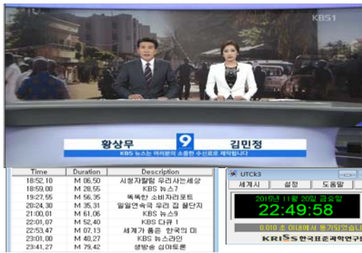
Fig. 8. Received picture(top) and EPG(bottom left), and reference clock from KRIS
