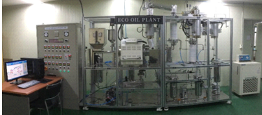
Fig. 3. Biomass pyrolysis system.
