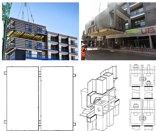
Fig. 5. Connection system of Unitised Building
