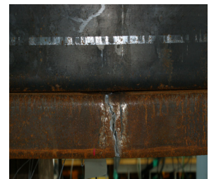
(b) ㄷ-Shaped bottom plate fracture
