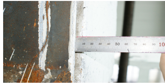
(d) Sliding between concrete and steel
