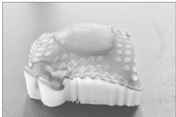
Fig. 5. Stereolithographic resin pattern and support material.
