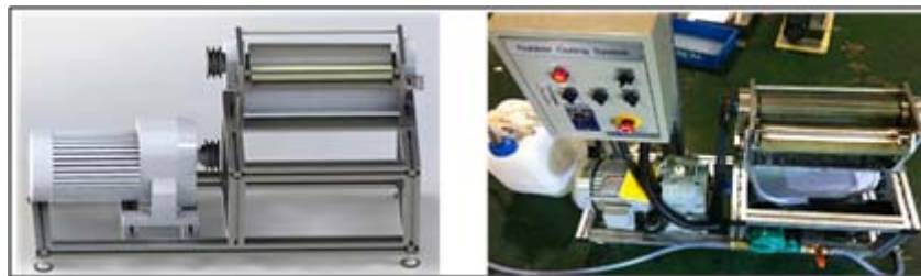
Figure 11. Design concept and manufactured machine by the result of Taguchi method
