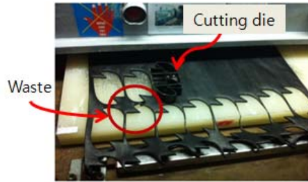
Figure 2. Rubber plate cutting with Cutting die
