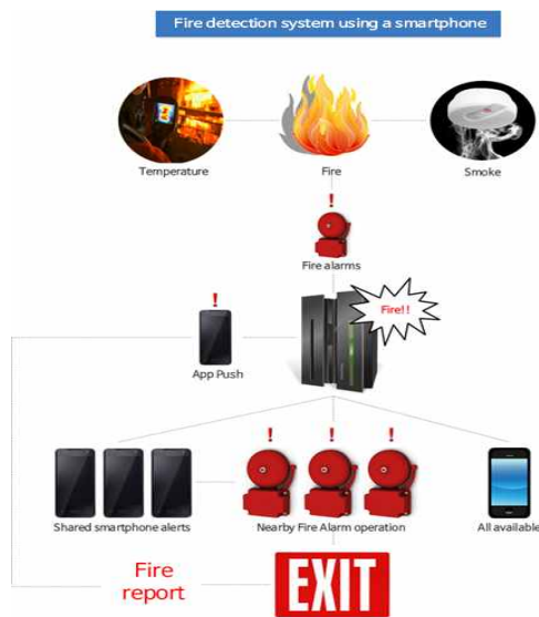
Fig. 1. A fire escape system using a smartphone
