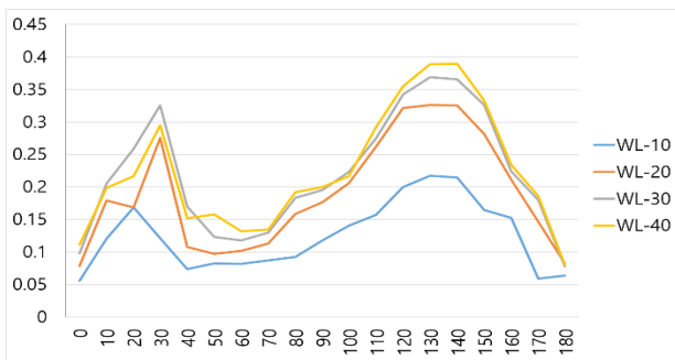
Figure 5. Pattern of Indoor Wind Flow - 1 (Wind Louver 10-40°)
