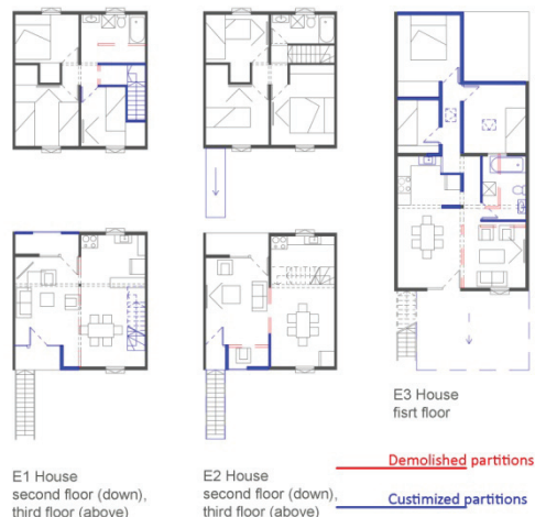
Figure 10. Three customized houses of Elemental Lo Espejo
