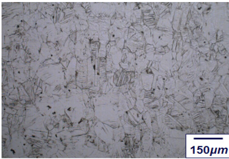
Fig. 2 Optical micrograph of 28% cold rolled Fe-26Mn-3Co-2Al damping alloy
