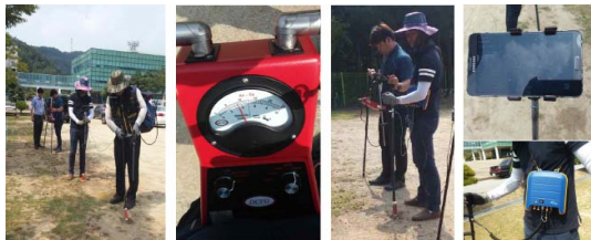
Fig. 17. Test of defect detection by using an analog DCVG and the developed DCVG.
