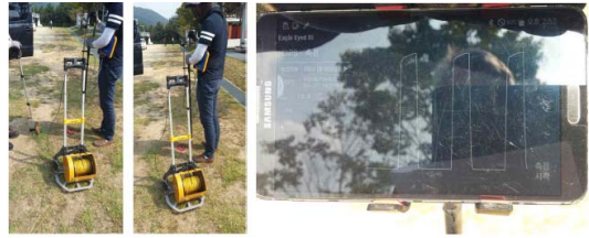
Fig. 20. CIPS by using a developed equipment (left and middle of the picture) and monitor readings (right side picture).
