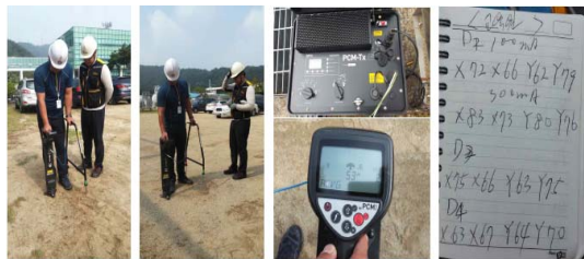
Fig. 16. Test of defect detection by ACVG.
