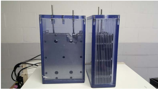
Photo. 2. DC type cell for brown gas generation.
