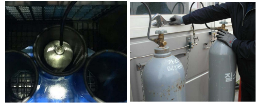
(1) Screwed an adapter after (2) Preparing nitrogen gas processing flow in seamless cylinder
