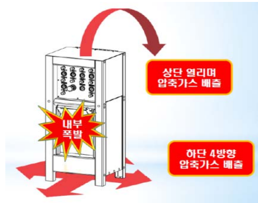
Fig. 5. The structure for solving overpressure when internal explosion in the safety cabinet for respiratory high-pressure cylinder.
