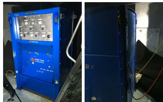
Fig. 8. Bursting test figure of the safety cabinet for respiratory high-pressure cylinder.
