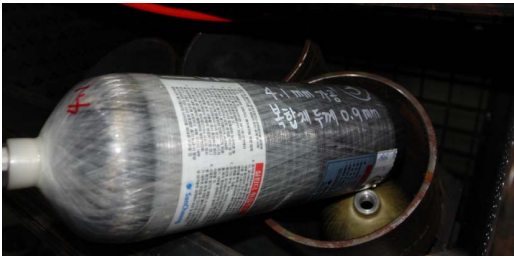
(1) Screwed an adapter after processing flaw in composite materials cylinder
