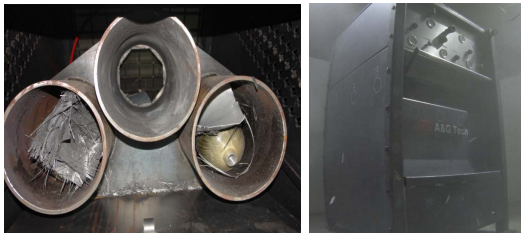
(2) Composite cylinder and Safety Cabinet after rupture
