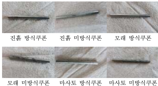
Fig. 8. corrosion coupon and pipe line buried site.
