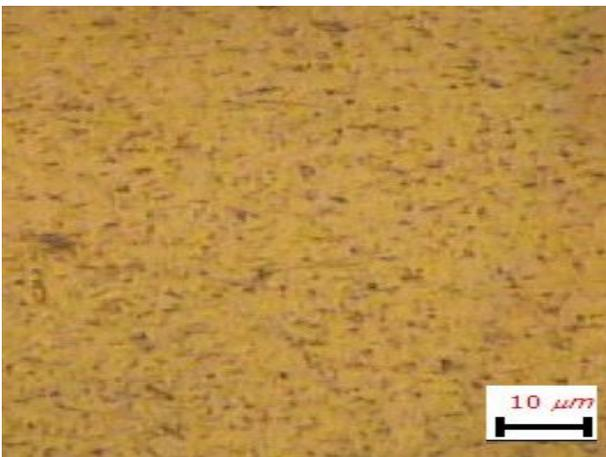
Fig. 16. Microstructure for 650°C 16hrs.
