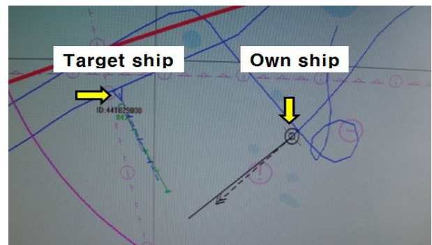
Fig. 4. Snap-shot of AIS screen in experimental situation showing the encountering angle of 135 degrees.
