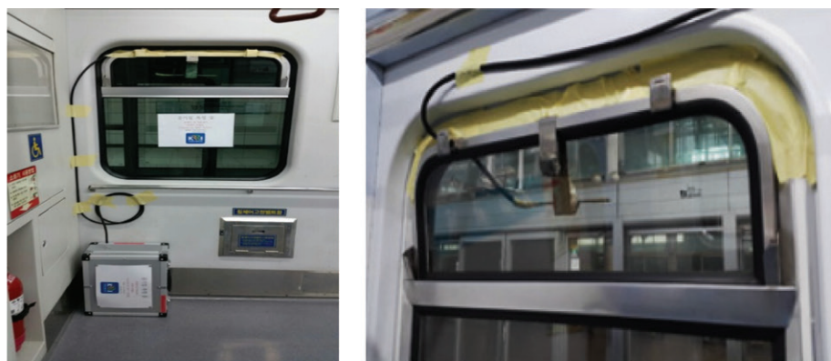
Fig. 2. Photos for a sampling location (left) and an inlet tube (right) in a subway passenger cabin.
