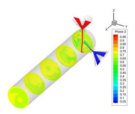
**Figure 6.** Contours of void fraction for resign phase (Phase 2) in different position in mixing head; Mixing ratio and nozzle diameter are 100:35 and 0.45mm, respectively.
