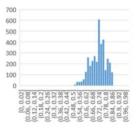
**Figure 10.** Histogram of void fraction for resing ar the outlet of mixing head; the mixing ratio and nozzle diameter are 100:35 and 0.3mm, respectively.
