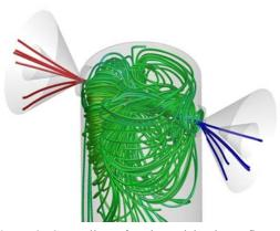
**Figure 3.** Streamline of resin and hardener flow inside the mixing chamber (The red, blue and green color signifies the resin, hardener and mixture of them, respectively).
