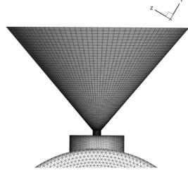
Figure 2. Nozzle geometry and structure mesh.
