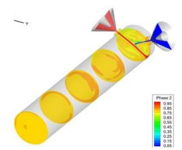
**Figure 5.** Contours of void fraction for resign phase (Phase 2) in different position in mixing head; Mixing ratio and nozzle diameter are 100:35 and 0.3mm, respectively.
