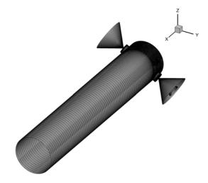
Figure 1. Overall view of computational domain. Two distinct nozzles are connected to a chamber.
