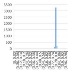
**Figure 8.** Histogram of void fraciton for resing ar the outlet of mixing head; the mixing ratio and nozzle diameter are 100:35 and 0.3mm, respectively.
