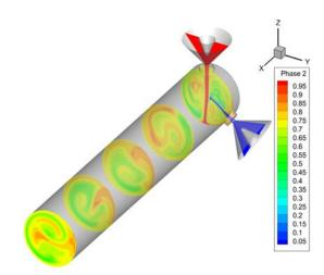
**Figure 7.** Contours of void fraction for resign phase (Phase 2) in different position in mixing head; Mixing ratio and nozzle diameter are 100:35 and 0.6mm, respectively.
