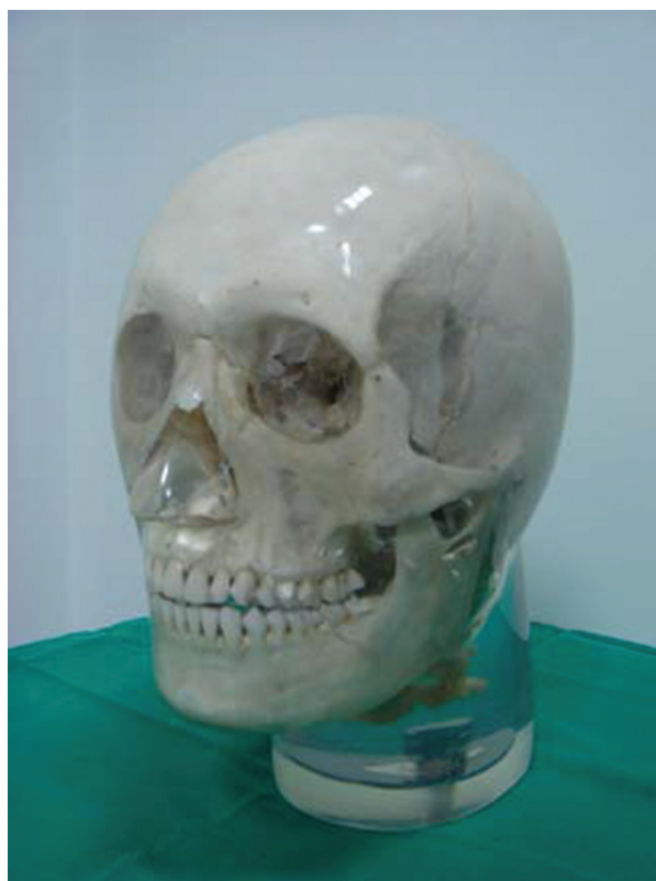
Fig. 1. Transparent X-ray skull phantom with a soft tissue replica.
