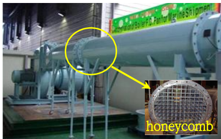
Fig. 5 Experimental setup for fan test
