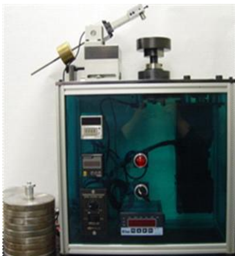
Fig.3. Pin-on-disc wear test system
