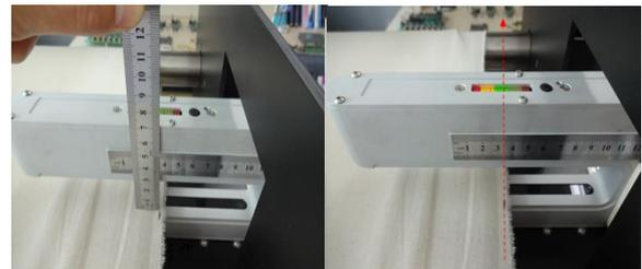
Fig. 10 Selvage sensing test
