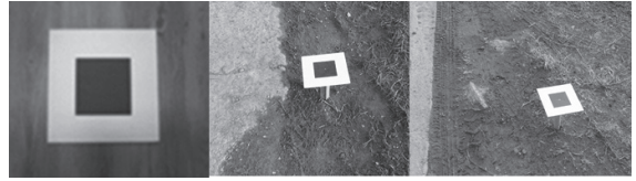
Fig. 6. Aerial target(left) placed at road slope(middle) and footpath of rice field(right)
