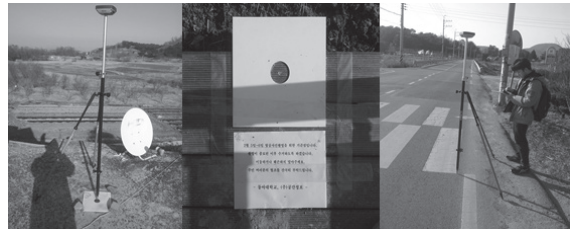
Fig. 3. GCP surveying and air target
