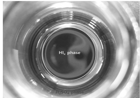
Fig. 5 Plane photograph of vial with Bunsen products; Cored HI x phase and H 2 SO 4 phase attached inner wall of vial
