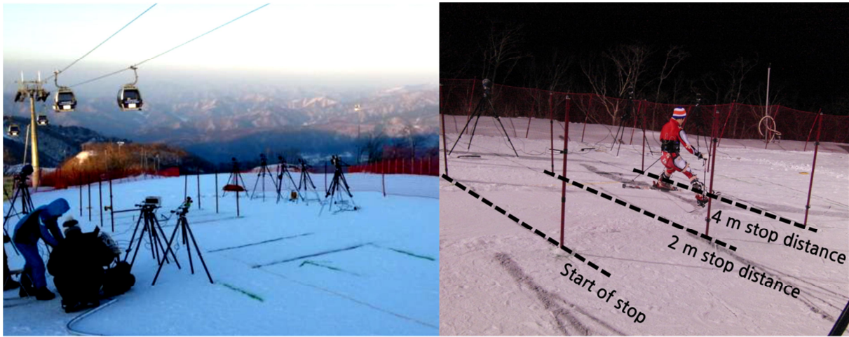
Figure 1. Experimental setup (left) and the two different snowplow braking distances (right).
