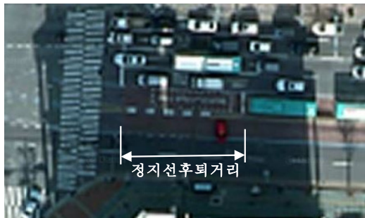
<Fig. 3> Operation case of turn lanes in median exclusive bus lanes
