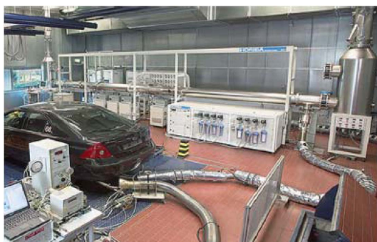
Fig. 1 Chassis dynamometer facility for measuring motor vehicle emissions
