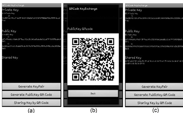
Fig. 5. Secure key exchange: (a) user's private key and public key, (b) QR code of the user's public key, and (c) after secure key exchange and generation of the shared key.
