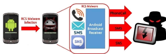
Fig. 1. Remote Control System (RCS) malware operating procedures.
