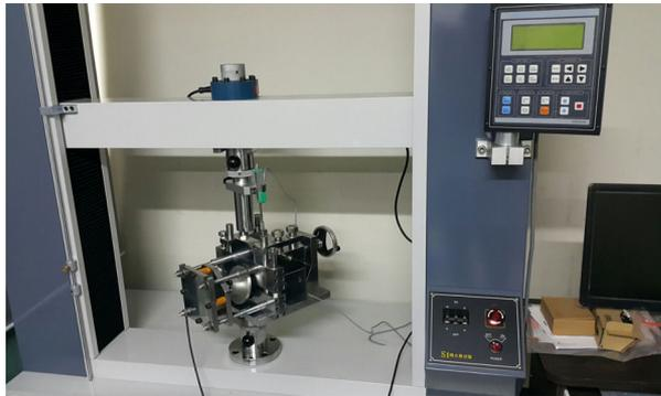
Fig. 3 Test Machine for Direct Shear Test
