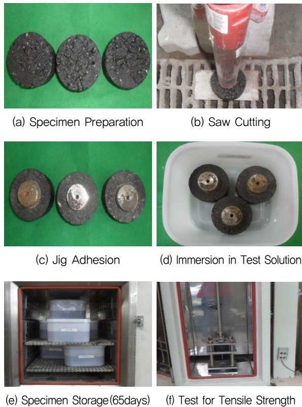
Fig. 3 Test for Surface Tensile Strength of Asphalt
