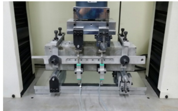
Fig. 3. Evaluation of flexural performance for HFRC
