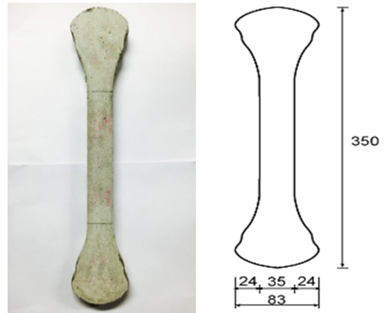
Fig. 1. Detail of the specimens for direct tensile test
