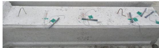
Fig. 7. Instrumentation for strain gauges
