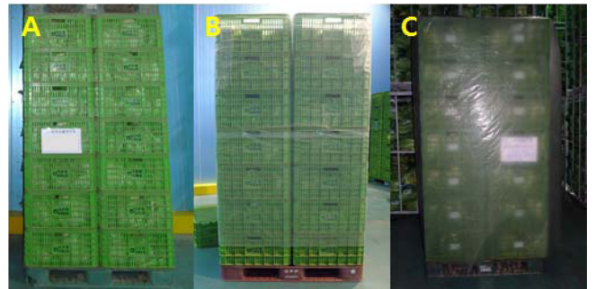
<Figure 2> Appearance of Pallet-unit MAP Treatment A, control; B, HDPE film; C, LLDPE F-film
