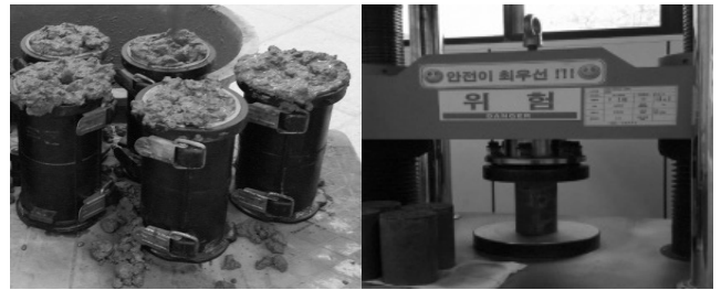
Fig. 3. (a) Preparation of concrete samples and (b) compressive strength measurement.
