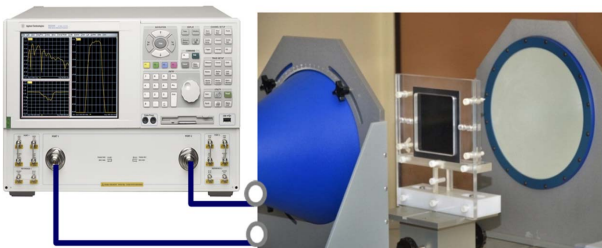
Fig. 4. Measuring system for electromagnetic properties (Free-space Measurement System)
