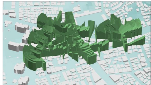
FIGURE 15. Result of computing about CCTV view area at all new locations
